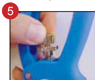
Turn dosing adjustment screw to set the required dosage. Retighten lock nut
